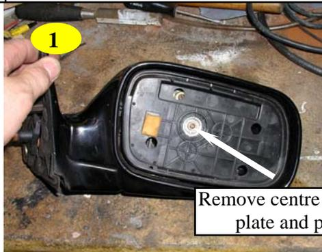
Remove centre pivot and put mirror back plate and parts somewhere safe!
