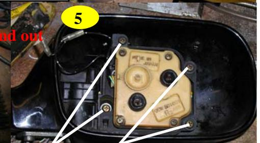
Remove 4 screws fixing cowl to folding/adjusting mechanism and wangle free so that you have now access to the pivot/motor cover
