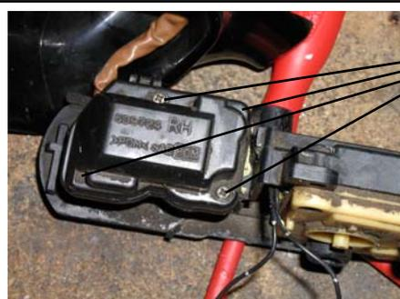
Remove the securing screws, pull off the plastic motor/gearbox cover and put the cover and screws in the same safe place that you have used to lose all the other small parts in to annoy you later on! - these screws also secure the folding motor
