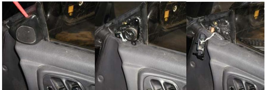
To remove the door card (need to do this just to get to the wiring for the mirror). 1- pop off the 3 screw covers and remove screws. 2- lever the door card off from the bottom and pull outward and upwards remembering to catch the fixing at the front that will fly off.
